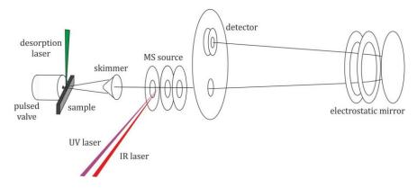
The set-up is designed to record conformation-selective IR spectroscopy of flexible molecules. Conformations are sorted according to their UV spectroscopic signatures, which are then used to select conformations for the next step, i.e., the IR/UV double resonance spectroscopy. The IR spectra obtained enable us to document the intramolecular interactions that stabilize the structures, by comparison with quantum chemistry calculations.
